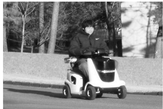
図10 歩行困難者用電動椅子 (スズキ セニアカー) Fig.10 Electric wheel chair for disabled people (Suzuki senior car.)
